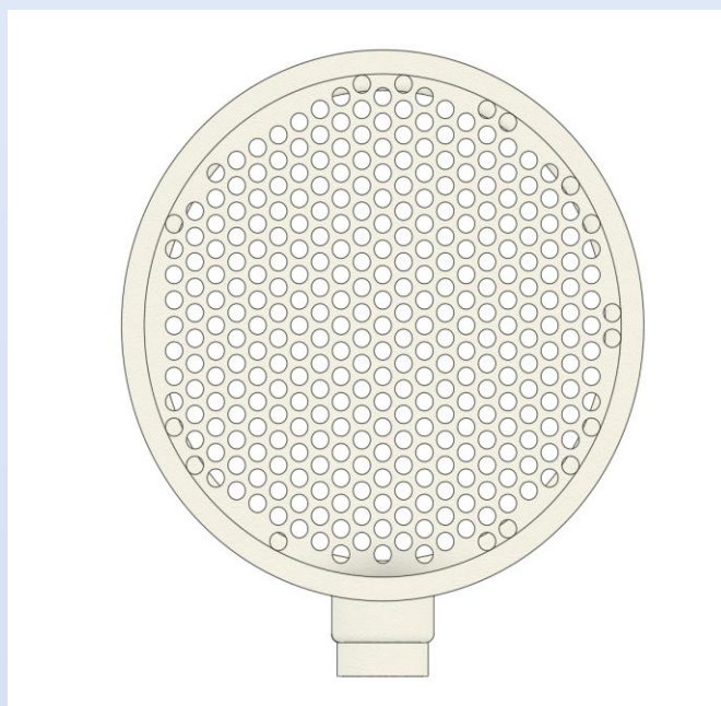
Figure 1(b): Circular plate with 329 micro-orifices ( \varnothing 0.8–1.1 mm) providing uniform flow conditioning and sensitive \Delta P at low flows.
